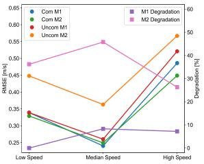
Fig. 8. The RMSE of the filtered speed using compensated model and uncompensated model. The circle represents the speed RMSE, while the square represents the degradation rate. Com denotes that all the IMU sequences are well compensated in training and testing, while Uncom denotes no compensation. The degradation rate is defined as (Uncom-Com)/Com. The uncompensation is only for the IMU biases, and the mounting angles are compensated for all sequences in this test.
