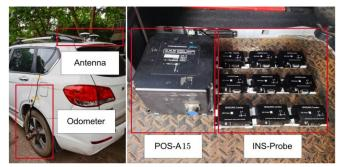
Fig. 3. Photograph of the test vehicle and system setup inside and outside the vehicle.
