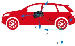
Fig. 2. Definitions of the vehicle frame (v-frame) and the IMU body frame (b-frame), and illustration of the IMU mounting angles and the lever-arms with respect to the v-frame.
