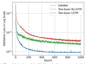
Fig. 6. The validation loss of the OdoNet and other two networks during the training. The loss is in log scale. The Bi-LSTM based network and LSTM based network have the same structures with OdoNet, except the four-layer 1D CNN network. Each layer of the Bi-LSTM has 64 nodes, and each layer of the LSTM has 128 nodes.
